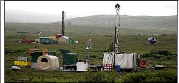
Workers drill test holes at the Pebble Partnership mining site near Bristol Bay, Alaska, in July 2007. (By Al Grillo -- Associated Press)
