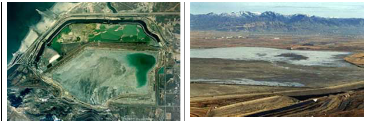
Figure 1. Kennecott Bingham Canyon Mine in Utah. (Left) Tailings impoundment (roughly 9,000 acres) with the Great Salt Lake at the top left. The pit is 0.75 miles deep, 2.5 miles wide, and covers 1,900 acres. (Right) Tailings are shown in the foreground (grey) with Salt Lake City in the background. Operations produced a 60 square-mile groundwater plume under valley to right, mostly from waste rock seepage. As of 2006, Kennecott had spent $370 million on cleanup and source control, and will be required to pump and treat aquifer water for at least the next 40 years. By 2009, 2.7 billion gallons of water will be treated annually to supply homes unable to use the aquifer.
